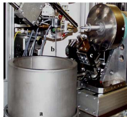
Figure 1 Diffraction set-up and crystal mounting robot with the dewar (a), plucker (b) and gripper (c).
